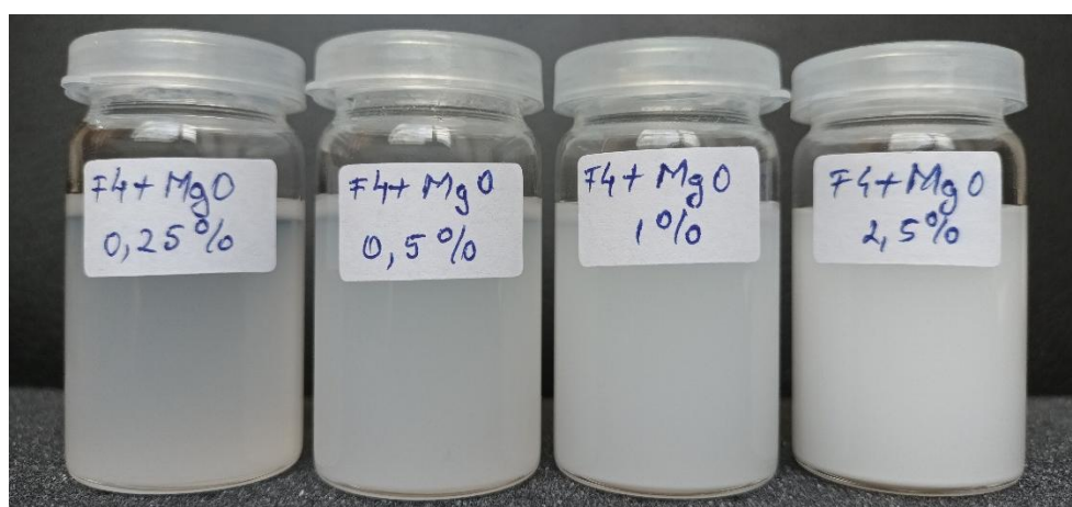
Figura 5. Nanofluidelile F4 + MgO, after 48h
